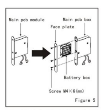
(5) As figure 5: Part the Main pcb into Face plate, Battery box and Main pcb box.
