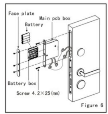
(6) As figure 6: Part the Main pcb into Face plate, Battery box and Main pcb box. Connect the cables of Reader, mortise and Main pcb box. Put the Main pcb box into door along with the cables, fix with screws. Place batteries in Battery box, put into the Main pcb box, fix the Face plate with screws.
