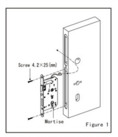
(1) As figure 1: Lead the nylon cable tie in the inclined hole and reach out the end of the nylon cable tie, then encircle the cable of Mortise, pull over to the top hole. Mount the Mortise on the door and fix it with screws.
