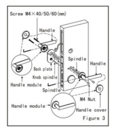
(3) As figure 3: Part the Handle modules into Handle covers and Handles. Loose the screw from handle by allen key (till Spindle able to insert). Put the Spindle and Knob spindle in the Mortise, then fix the Handle and Back plate with screws and nuts (M4 $\times$ 40 for 35-45 door thickness, M4 $\times$ 50 for 45-55, M4 $\times$ 60 for 55-65). Tight the screw from Handle with allen key, mount the Handle cover at last.
