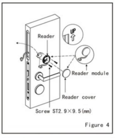
(4) As figure 4: Part the Reader module into Reader cover and Reader. Let the cable get through the door leaf and stretch out from the side hole, fix the reader with screws (mind the arrow upwards), then mount the reader cover.
