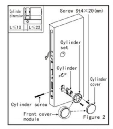
(2) As figure 2: Rotate to part the cover modules into Cylinder sets and cylinder covers. Insert Cylinder into mortise and fix with cylinder screw. (If customer prepare cylinder themselves, please make sure the size of cylinder is the same with the dimension above) Then use the corresponding screws to fix the Cylinder sets, mount the cylinder covers.
