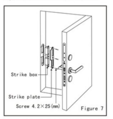
(7) As figure 7: Install the Strike box and Strike plate on the door frame, fixed with screws. Check if lock and mortise works properly by using cards to open.
